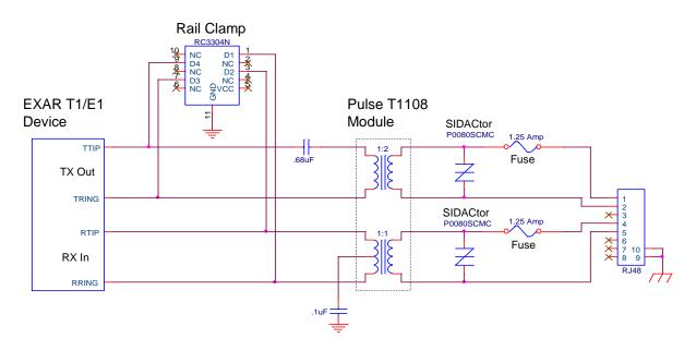
Figure 2. Reference Schematic for GR-1089 Protection – Applications Without Power Feed on Twisted Pair
