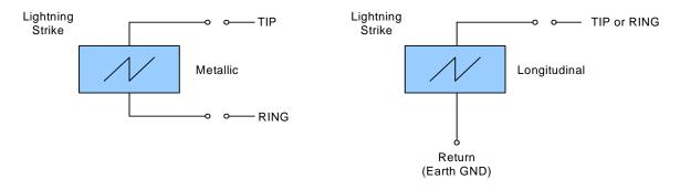
**Figure 1. Metallic and Longitudinal Modes**
