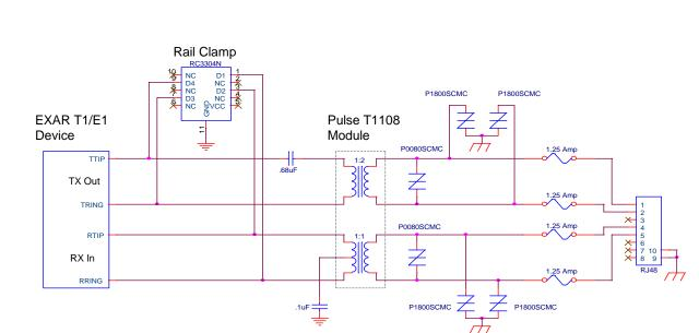
Figure 3. Reference Schematic for GR-1089 Protection – Inter-Building Applications With Power Feed on Twisted Pair
